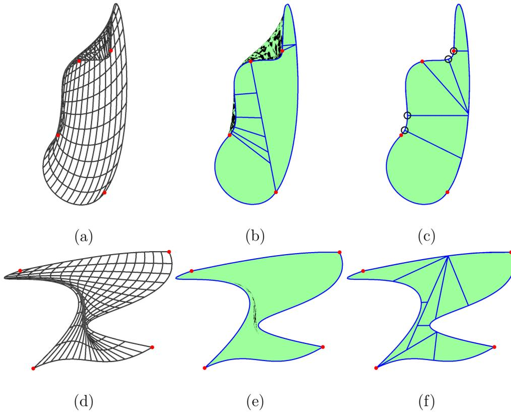
Figure 9: Degeneracy in a Coons patch. The dots indicate corner control points (nodes) and the open circles indicate the points of greatest degeneracy on the boundary, as determined by the quartic root solver: (a) overlapping isoline mesh; (b) overlapping patch; (c) nonoverlapping subpatches; (d) internally degenerate isoline mesh; (e) internally degenerate patch; (f) nondegenerate subpatches.
