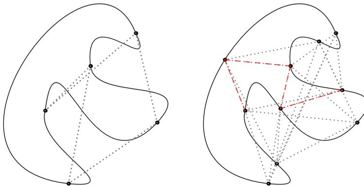
Figure 2: The left-hand figure illustrates a case where all line segments between nodes separated by two or three segments (dotted lines) are rejected in the **bezulate** algorithm. The right-hand curve shows that several connections (dashed red lines) become possible upon subdivision.
