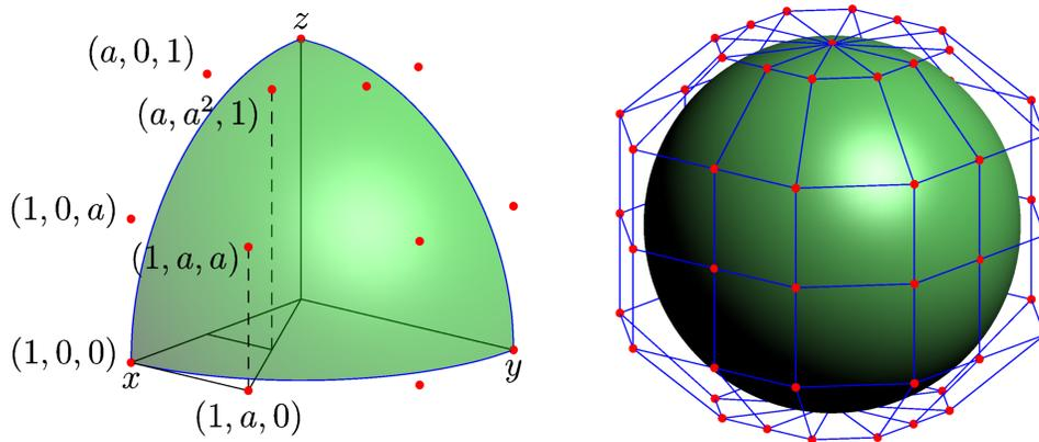
Figure 8: Bézier approximation to a unit sphere. The red dots indicate control points.
