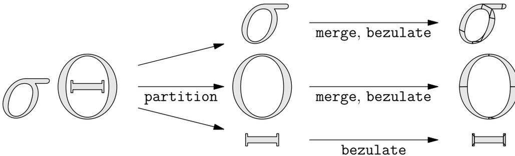
Figure 4: Illustration of the `partition` algorithm. The five curves that define the outlines of the Greek characters  $\sigma$  and  $\Theta$  are passed in a single array to `partition`.
