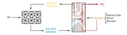
Capturing  $CO_2$  directly from the air allows emissions originating from any source to be managed with standardized, scalable industrial facilities. Carbon Engineering's full-scale design, for example, could absorb the emissions created by 300,000 typical cars.
