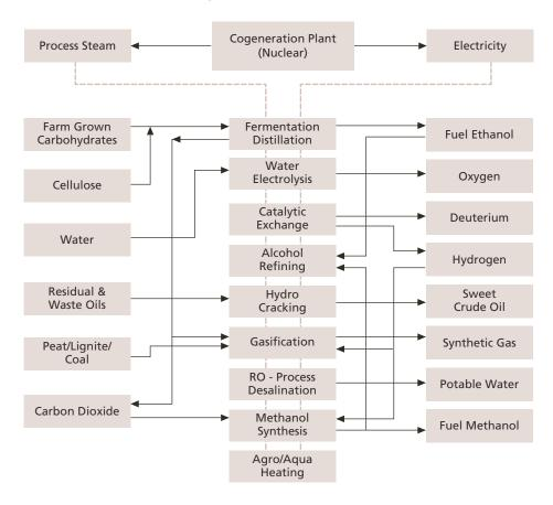
Steam from Bruce nuclear plant could be diverted to the BNGS bulk steam supply system to provide energy for the production of heavy water, to heat buildings within the development, and to provide energy for industries at the Bruce Energy Centre at the boundary of the site. One of the largest bulk steam systems in the world, this system was capable of producing 5,350 MW of medium-pressure process steam from the reactors' high-pressure process steam (CNWC, 2014).
