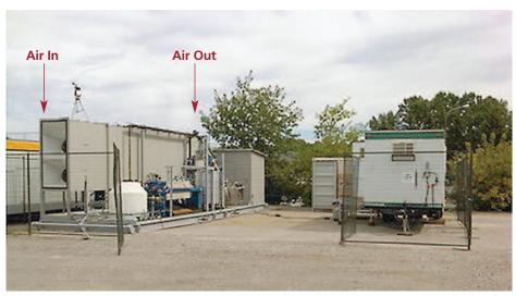
Carbon Engineering's air capture prototype uses an oxy-fuel natural gas kiln to drive the  $CO_2$  out of the solid calcite.
