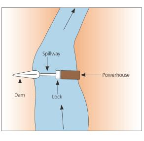
Here again, due to swift currents, a narrow riverbed and high shorelines, the complex' final downstream dam is located approximately 15 kilometres upstream of the village of Artic Red River (Figure 10). Site construction requires two phases, the first focusing on spillway construction, so that the river can subsequently be diverted to build the powerhouse. The 22 metre head is harnessed by
