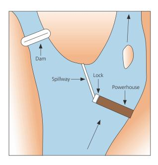
At the present time, there is no village or road access at this site. Even so, the site is recommended in order to minimize flooding. Steep shorelines and the presence of an island make this an ideal site (Figure 7). Diverting the river initially on its west branch enables the project site (i.e., for both powerhouse and spillway) to be enclosed by cofferdams, and built in a single phase upstream of the island. Following this, the spillway is used to divert the river while a
