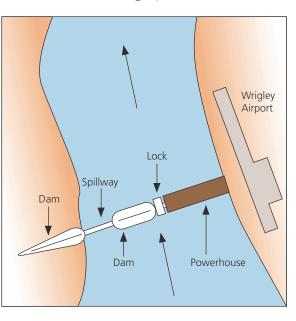
Immediately facing Wrigley airport, even though river width is insufficient to build both powerhouse and spillway in a single construction phase, this site is recommended to avoid local flooding (Figure 6). The spillway, capacity 46,000 CMS, is located on the west side of the river and is built in the initial construction phase. The next phase consists of the construction of the powerhouse on the east (i.e., right) side of the river, consisting of 19 generators and
