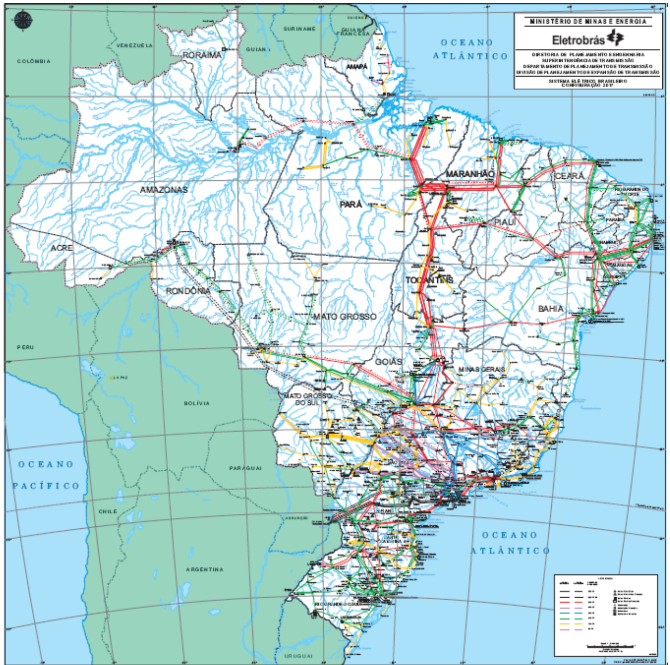
Figure 4-7: Brazil's national grid (as projected for 2017)
