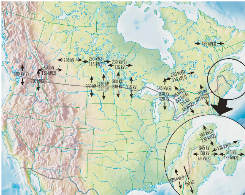
Source: National Energy Board, Canadian Electricity Exports and Imports: An Energy Market Assessment, January 2003, p. 9. The numbers indicate the voltage of the power lines from each province to adjoining provinces and the states. If there is more
