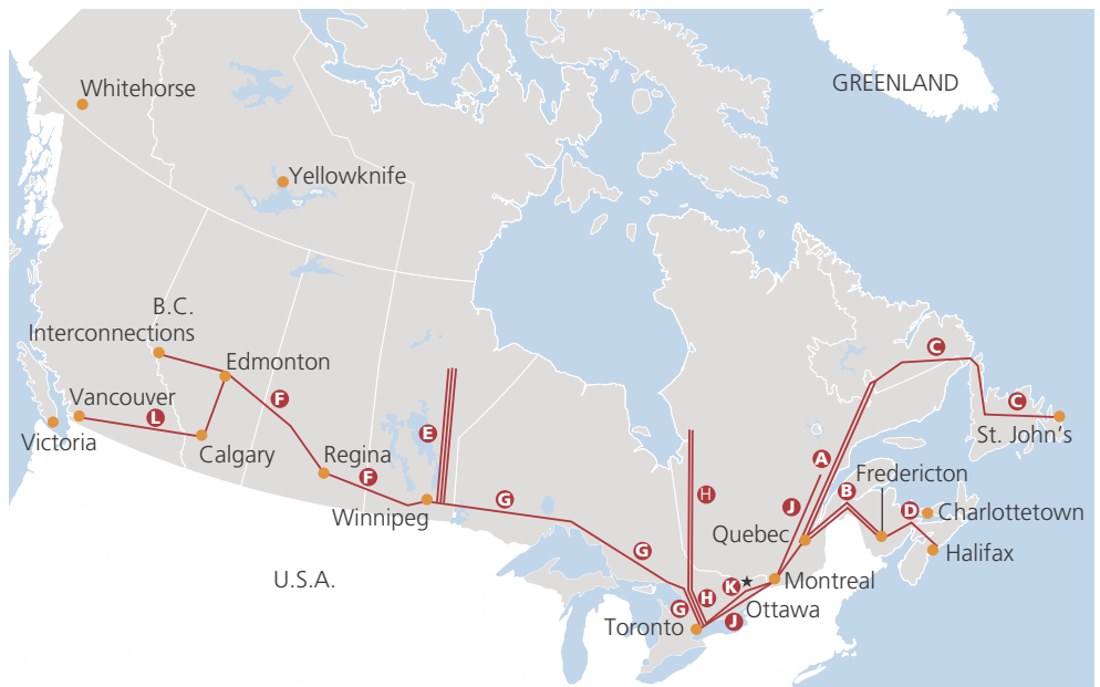
Figure 6 Illustrative 735 kV Pan-Canadian Transmission and Interconnection Scenario*
