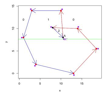
Figure 3: Both methods mark vertex A inactive but differ on the value of the turning number.
