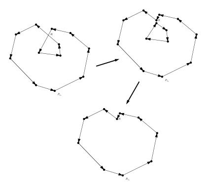
Figure 9: Clipping an internal loop
