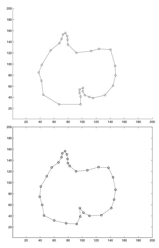
Figure 15: The top figure gives an example of propagated vertices, and the bottom figure shows equidistribution of vertices via a curvature based monitor function. Notice that there is some inherent smoothing due to the interpolation.
