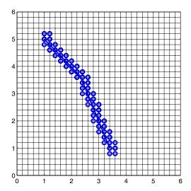
Figure 17: Nodes surrounding a barrier where the propagation speed is set to zero.
