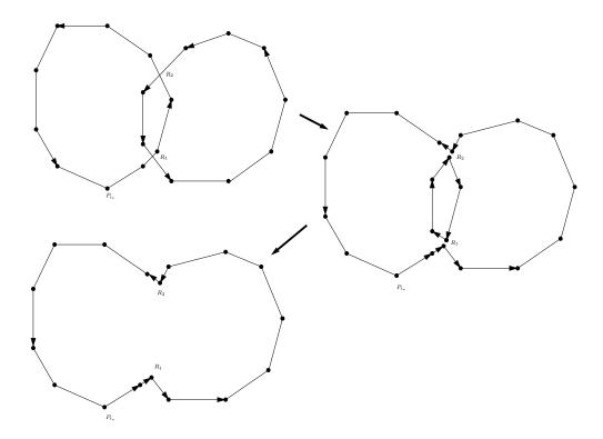
Figure 11: Merging of two simple fire fronts
