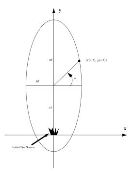
Figure 1: The elliptical shape of fire growth from a point at time t.
