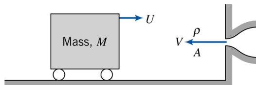
Figure 2: Rectangular block moving toward nozzle.
