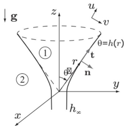
**Figure:** Cone set-up in spherical system of coordinate;  $\theta^*$  is the cone semi-angle.
