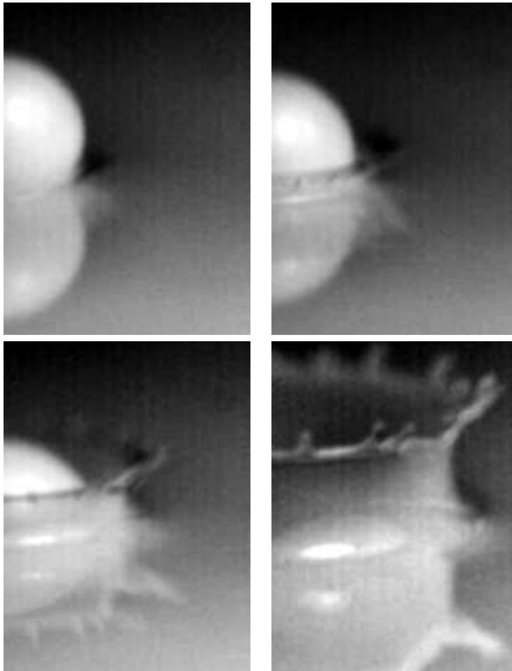
From ejecta to crown; time interval  $t = 1610 \mu\text{s}$ .
