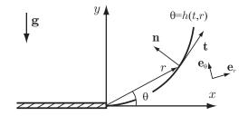
FIG. 2. Near the plate edge region:  $\theta = -\pi$  is the plate and  $\theta = h(t,r)$  is the liquid interface.
