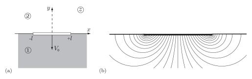
FIG. 1. Plate impact problem: (a) setting, and (b) flow field.
