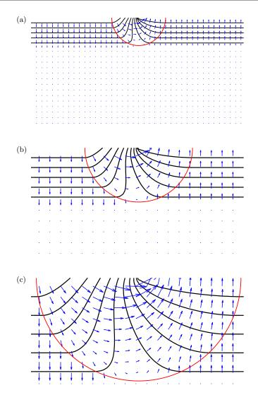
FIG. 6. Equipotential patterns (black lines) of (83) and velocity fields (blue arrows) near the plate edge at three different times: (a)  $t = t_1 \ll l/c_0$ , (b)  $t = 2t_1$ , and (c)  $t = 4t_1$ ; the half-circle shows the boundary of the disturbance and its center corresponds to the plate edge. The scaling self-similarity of panels (a)–(c) suggests self-similarity of the solution near the edge at early times.
