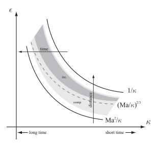
FIG. 3. Regions of validity of the inviscid incompressible (45) (dark shaded) vs the compressible (92) (light shaded) approximations for Ma  $\ll$  1. The time and distance arrows crossing the region indicate the growth of the corresponding variable (time or distance), cf. discussion in Sec. VI.
