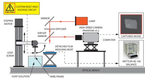
Figure 1: Schematic of experimental setup used for soap film experiments.
