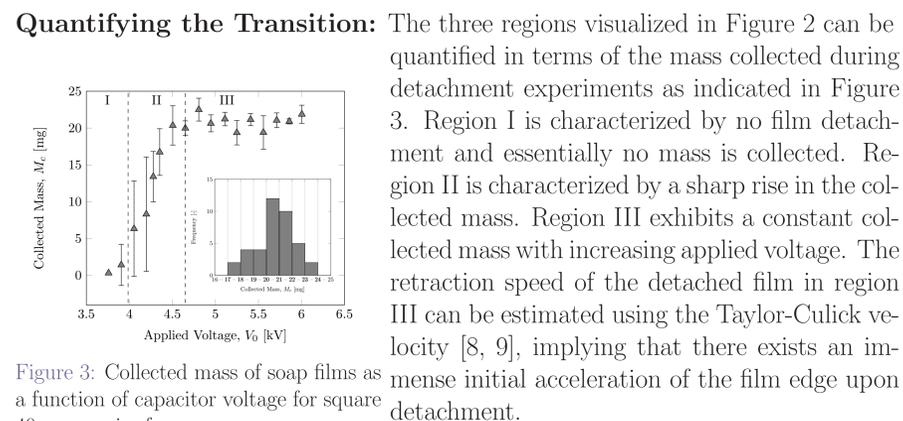
Figure 3: Collected mass of soap films as a function of capacitor voltage for square 40 gauge wire frame.
