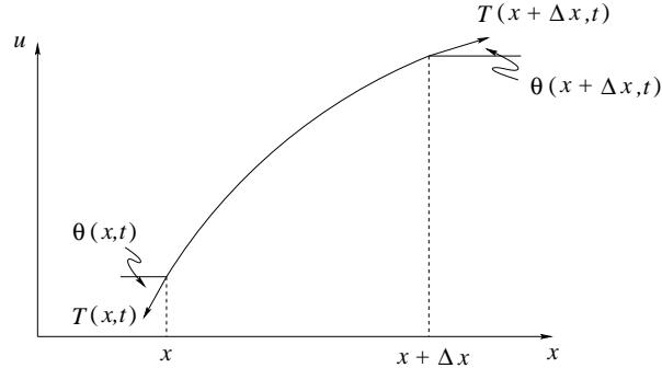
Applying Newton's second law to the small portion of the string between  $x$  and  $x + \Delta x$ , if  $\rho$  is the mass per unit length, we have
