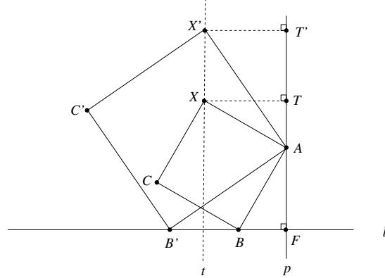
Now the construction is clear, given lines  $\ell$  and  $m$  and a point  $A$  not on  $\ell$  or  $m$ , drop a perpendicular  $p$  from  $A$  to  $\ell$ , hitting  $\ell$  at  $F$ . Next draw a line  $t$  parallel to  $p$  and a distance  $AF$  from  $p$ , hitting  $m$  at  $D$ . Now that the side  $AD$  of the square  $ABCD$  has been constructed, we erect a perpendicular from  $A$  hitting  $\ell$  at  $B$ , and then erect perpendiculars from  $B$  and  $D$  intersecting at  $C$ .
