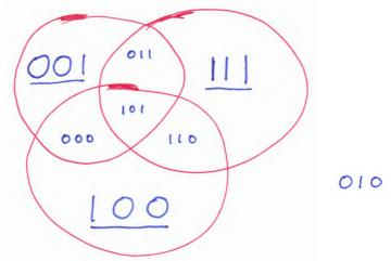
Since in the above code each pair of codewords has a Hamming distance of 2 we can detect 1 error.
