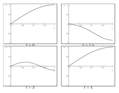
The solution is periodic in time with period 4 time units. The solution is shown below for t = 0, 1.5, 3 and 4, respectively.
