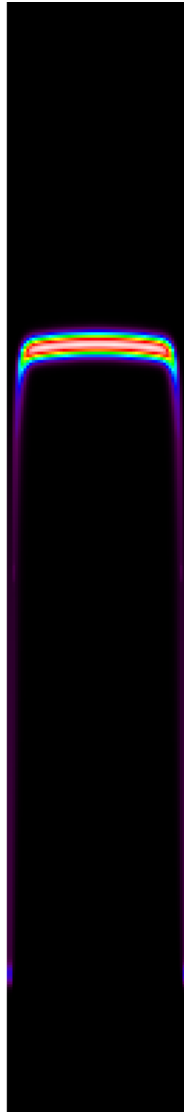
Figure 4.19: The concentration field advected by an electro-osmotic flow and a pressure-driven flow. Black corresponds to 0 and white corresponds to 1.
