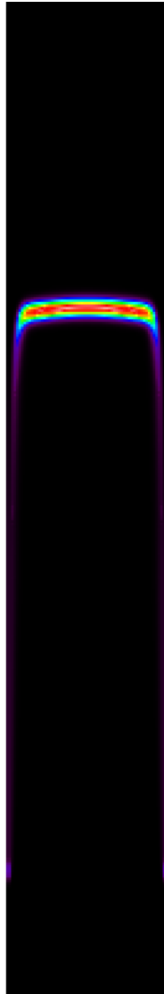
Figure 4.21: The concentration field in simulation (c) advected by a flow, where the pressure effect is neglected explicitly. The resulting violation of incompressibility produces spurious results. Black corresponds to 0 and white corresponds to 1.2.
