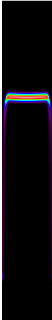
Figure 4.20: The concentration field advected by a pure electro-osmotic flow. Black corresponds to 0 and white corresponds to 1.
