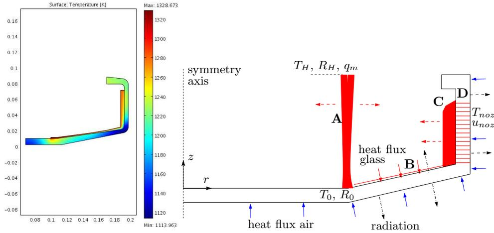
FIGURE 2. Melting phase. *Right*: Sketch of melt distribution (red) in the disk. A – glass string entering disk from stove, B – thin glass film, C – glass reserve (free surface flow), D – perforated wall with capillaries (pipe flows of glass). *Left*: Simulation of heat transfer in disk and glass reserve.
