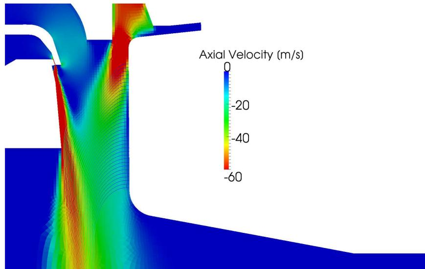
FIGURE 5. Final simulation result for glass jets and air flow. The color map visualizes the axial air velocity. In addition, immersed glass jet representatives are colored with respect to  $u$ .
