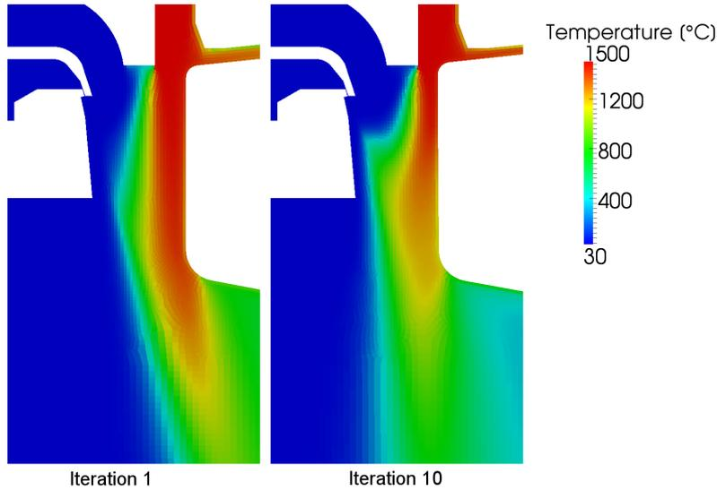
FIGURE 4. Air temperature in the iteration procedure of Algorithm 1. Zoom of the rotationally invariant flow in the region at the perforated disk wall.
