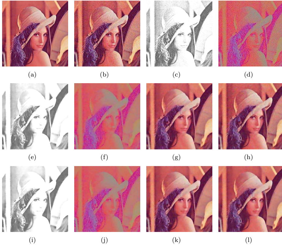
FIGURE 2. Color denoising based on CB color model. Image size is 256 \times 256 . (a) Original image. (b) Noisy image (SNR=5.1574). (c) The brightness component of noisy image. (d) The chromaticity component of noisy image. (e) Denoising result of brightness component using proposed algorithm (iter=10). (f) Denoising result of chromaticity component using proposed algorithm (iter=10). (g) Denoising result of noisy image using proposed algorithm (SNR=29.8560), t=1.147s ; \mu_1 = 0.008 , \lambda_1 = 0.065 , \mu_2 = 2 , \lambda_2 = 10 , \beta = 10 . (h) Denoising result based on RGB color model using proposed algorithm (SNR=29.5145), iter=10, t=0.878s ; \mu = 0.004 , \lambda = 0.04 . (i) Denoising result of brightness component using dual method [3] (iter=50). (j) Denoising result of chromaticity component using dual method [3] (iter=50). (k) Denoising result of noisy image using dual method [3] (SNR=28.2305), t=6.971s . (l) Denoising result based on RGB color model using dual method [3] (SNR=29.3835), iter=50, t=4.663s .
