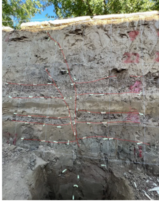
FIGURE 16. Field photograph of Songzhuang ground cracks (Beijing geological environment institute).
