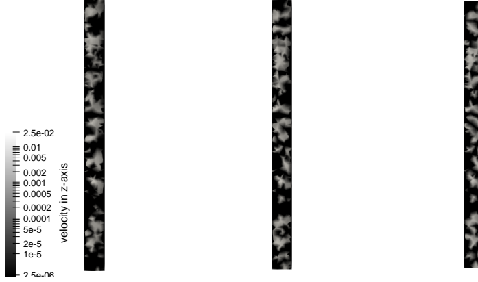
FIGURE 9. The velocity magnitude in the z -axis at t = 10 on a log scale ranging from 2.5e - 6 to 2.5e - 2 . In the figure from left to right: classical URANS models kinetic turbulence length scale and Prandtl, and 1/2-equation model. We observe that vertical rotations are consistent with irregular Taylor cells.
