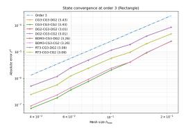
FIGURE 3. Convergence of  $\mathcal{E}^{\mathcal{X}}$  as a function of h at order 3, with the optimal choice of finite element families. See values in bold on Table 3.
