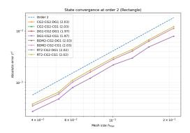
FIGURE 2. Convergence of  $\mathcal{E}^{\mathcal{X}}$  as a function of h at order 2, with the optimal choice of finite element families. See values in bold on Table 2.
