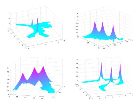
FIGURE 3. Biquadratic B-spline functions  $u^h$  approximating the exact solution (46) of Poisson equation for several regions. Top left: Havana bay, top right: Toba lake. Bottom left: V. de Bravo reservoir, bottom right: Grijalva channel.
