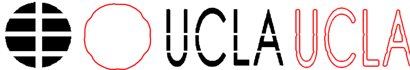
FIGURE 3. Segmentation results using Algorithm 1 . The 2nd and 4th images are the segmented contours of the 1st and 3rd images, respectively.
