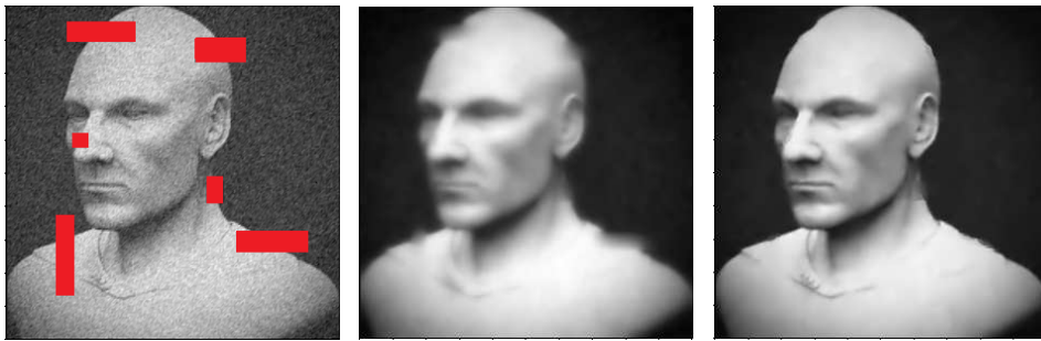
FIGURE 15. From left to right: Damaged and noisy - restored at iteration 5 - restored at iteration 20.
