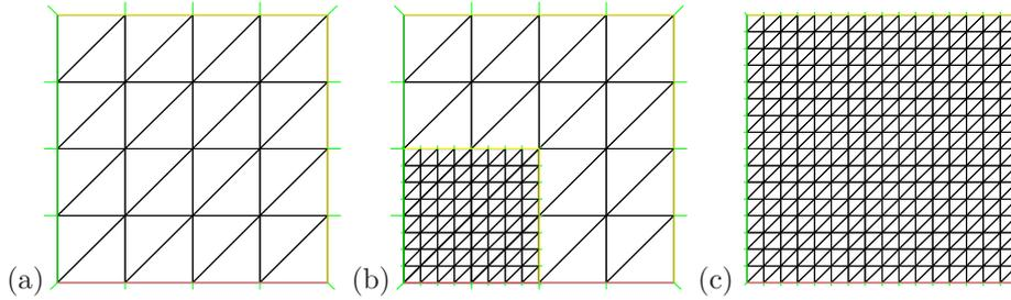
FIGURE 3. Meshes: (a) a global coarse mesh; (b) a locally refined mesh; and (c) a global fine mesh.
