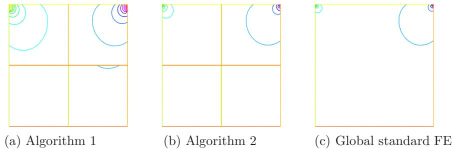
FIGURE 8. Contours of pressure  $p^h$  for the driven cavity flow: (a) Algorithm 1; (b) Algorithm 2 (it=20); and (c) global standard finite element method.
