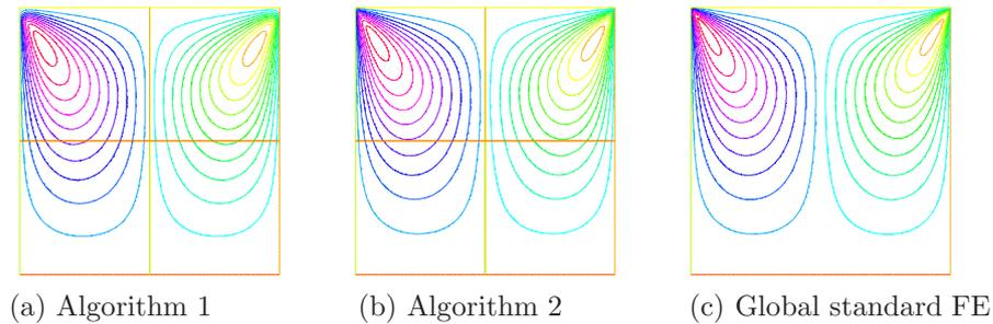
FIGURE 7. Contours of  $u_2^h$ -velocity for the driven cavity flow: (a) Algorithm 1; (b) Algorithm 2 (it=20); and (c) global standard finite element method.
