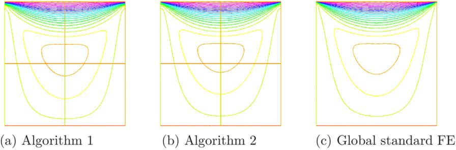
FIGURE 6. Contours of  $u_1^h$ -velocity for the driven cavity flow: (a) Algorithm 1; (b) Algorithm 2 (it=20); and (c) global standard finite element method.
