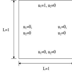
FIGURE 5. Lid-driven cavity flow.
