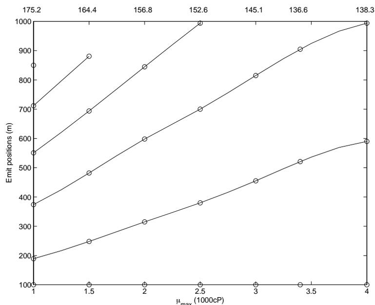
FIGURE 9: Position of the EMIT regions as a function of the maximum allowable viscosity,  $\mu_{\max}$ . Each value of  $\mu_{\max}$  considered has a corresponding production rate  $\eta(L)$ . These values are illustrated above their respective values of  $\mu_{\max}$ .
