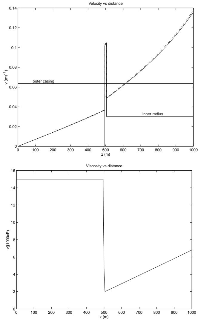
FIGURE 6: The velocity and viscosity as a function of distance along the wellbore. Again, where they are distinguishable, the shooting method solution is a solid line where the SOR method is indicated with a dot-dashed line. A longitudinal section of the wellbore is indicated in the plot of the velocity.
