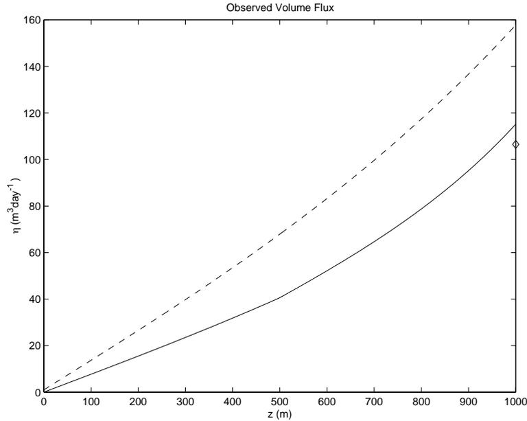
FIGURE 7: The production rate  $\eta_{sm}(z)$  as a function of distance along the wellbore for the simplified model. Only the production at the pump  $\eta_{cc}(L)$  was available from the CFD code and is indicated with the diamond. The dashed curve is the production rate for the case of no EMIT described in Section 5.
