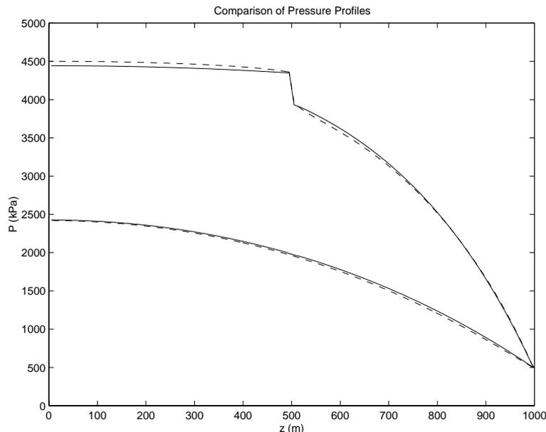
FIGURE 4: Comparison of the pressure profiles with the commercial code. Two cases are shown: (1) with no EMIT and (2) with an unpowered EMIT. The commercial code is indicated with a dashed line whereas our solution has a solid line. The upper curves correspond to the second case. There is good agreement between the two models.
