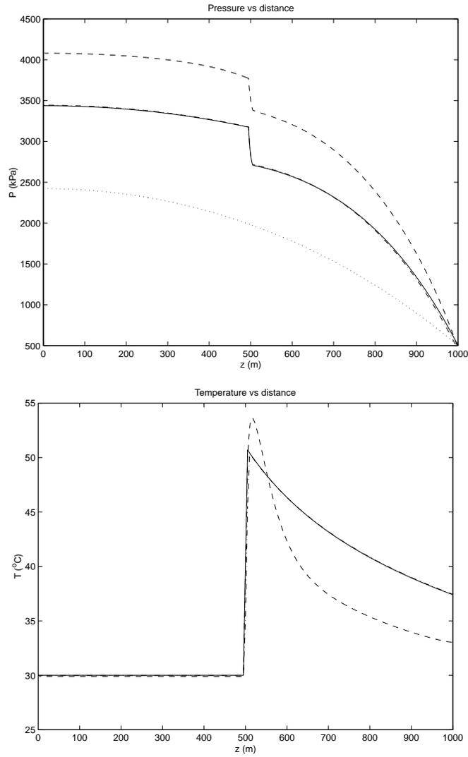
FIGURE 5: The pressure and temperature as a function of distance along the wellbore. For these, the CFD code was available, and are the dashed lines in the respective plots. More than one method was used to solve the simplified model. Where they are distinguishable, the shooting method solution is a solid line where the SOR method is indicated with a dot-dashed line.
