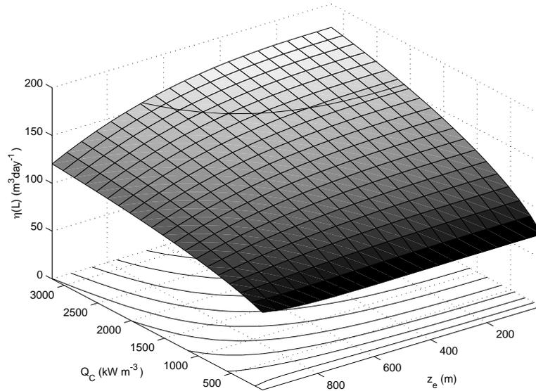
FIGURE 8: The production rate at the pump  $\eta_{sm}(L)$  as a function of the location of the centre of the EMIT,  $z_e$ , and the applied power. Rather than using the total power, we simply report the value of  $Q_c$ , the power in the casing. We have taken  $Q_e = Q_c/10$ . The contour on the surface is located at  $\eta(L) = 156.03 \text{ m}^3/\text{day}$  corresponding to the flux if there was no EMIT.
