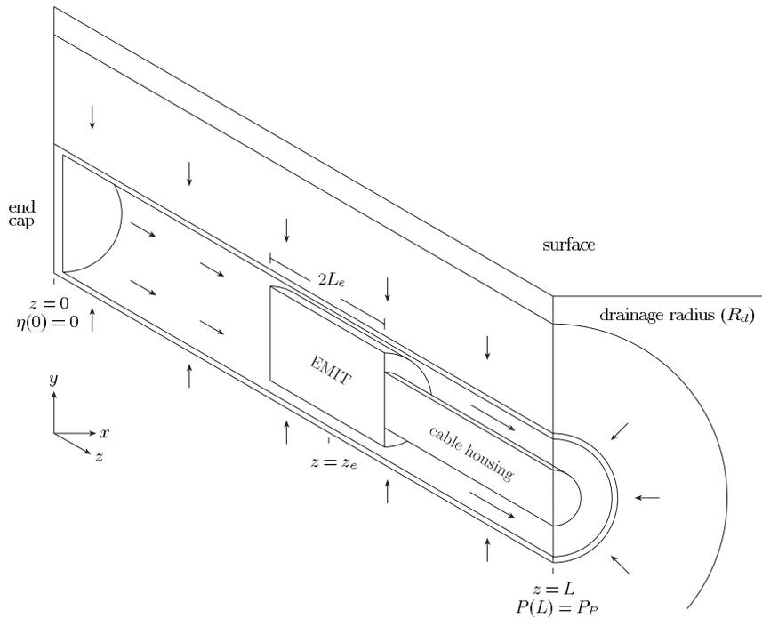
FIGURE 1: Cross section of the overall geometry for the horizontal wellbore problem. The rate and direction of the oil flow is indicated with the arrows. At  $z = 0$  there is an end cap and the horizontal flow is zero while at  $z = L$  there is a pump that maintains the producing pressure  $P_P$ .
