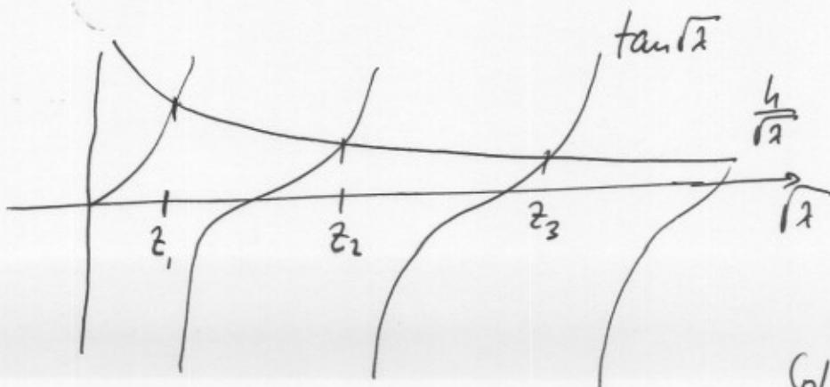
$$(b) \text{ for } n \text{ large : } z_n \sim (2n-1)^{\frac{n}{2}} \quad \Rightarrow \quad \lambda_n \sim \left(\frac{2n-1}{2}\right)^2 \pi^2 \text{ large frequencies of oscillation.}$$
