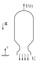
Figure 1: Rocket moving straight up.
