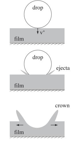
From ejecta to crown; time interval  $t = 1610 \,\mu s$ .
