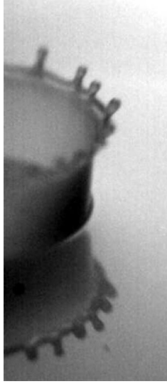
FIGURE 2. Example of accelerated curved liquid interface: drop splash on thin film.
