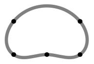
• First, linear equations involving the curvature are solved to find the direction through each knot. Then, control points along those directions are chosen:
